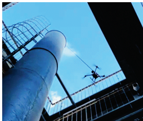
Fig. 4 Collecting smoke from a chimney using a gas chromatograph installed on a drone.
