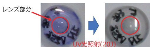
Fig. 3 Marker ink disappeared after UV radiation
