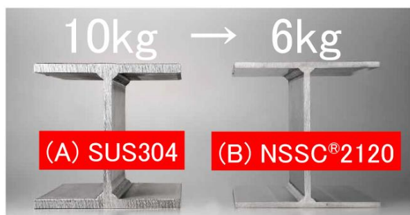
Fig.2 Thickness of H-section stainless steels, here austenite stainless steels of Type SUS304 (A) and new lean duplex stainless steels named NSSC2120 (B).
